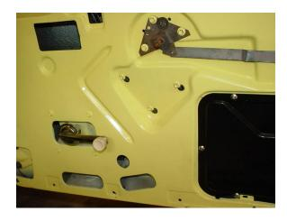
After tightening the screws restore the upper limit bracket to its original position. Now try out the window. By changing the position of the scissors you have increased the upper travel limits of the mechanism. This worked for me and I did not have to remove the glass or any of the mechanism to accomplish the modification.
